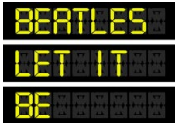
Figure 1. Scrolling is simulated by transmitting strings of text in shifted sets. The string above would display "BEATLES - LET IT BE."
